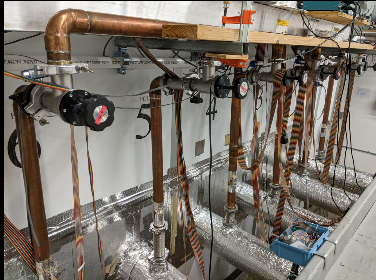
Image: Connection of FDL to current vacuum manifold
