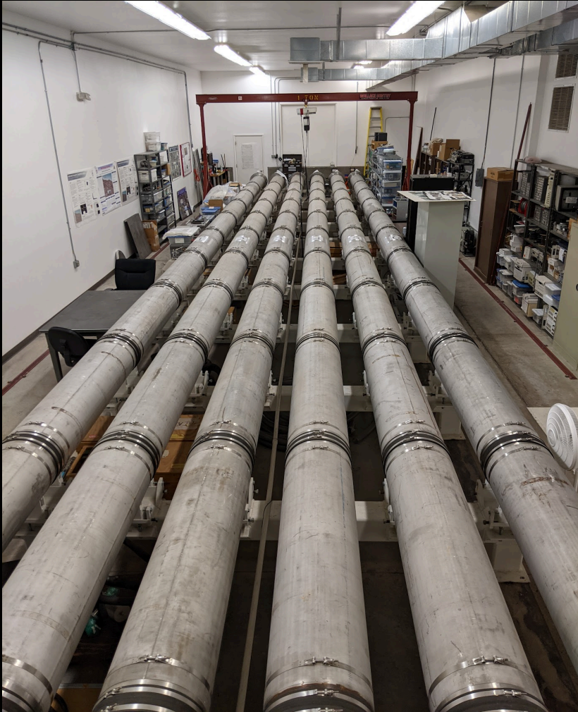
Image: The six fast delay line vacuum tubes
